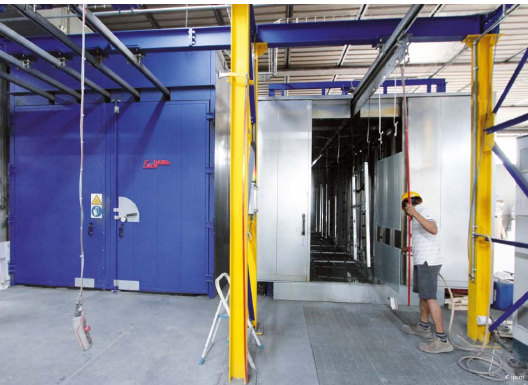
On the left the drying and/or curing oven and on the right the pre-treatment tunnel.
