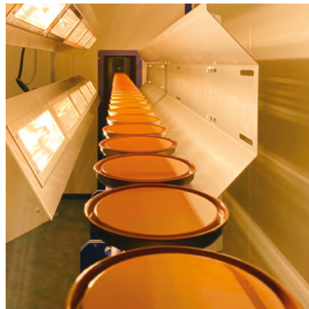
➤ Continuous automatic liquid painting systems with floor conveyor
