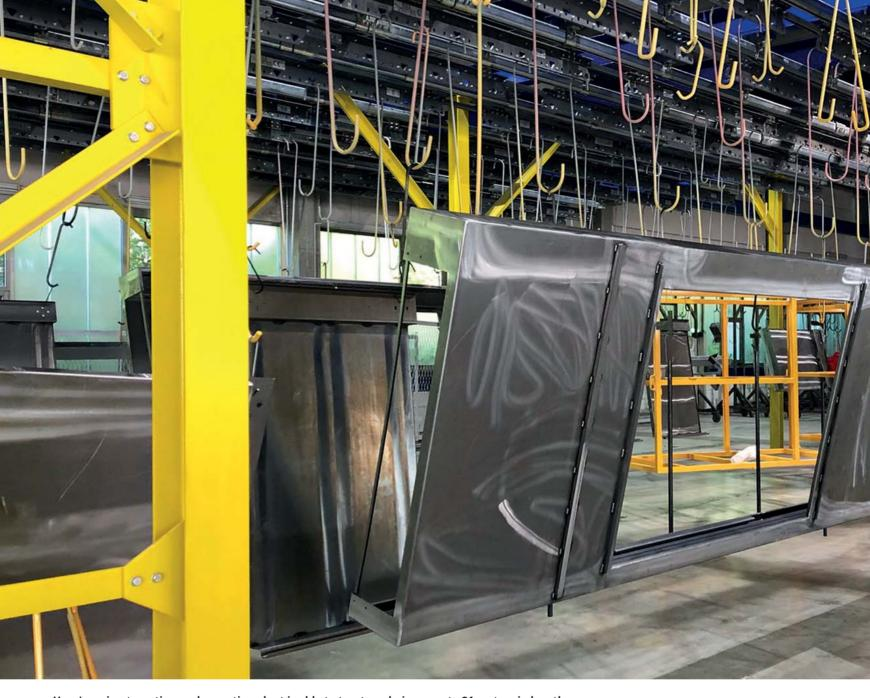
Haas' semi-automatic powder coating plant is able to treat workpieces up to 21 metres in length.
