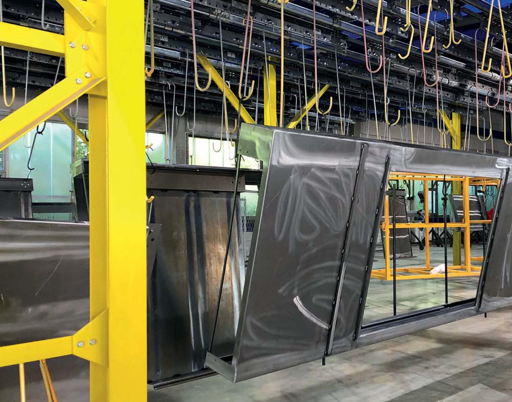
Haas' semi-automatic powder coating plant is able to treat workpieces up to 21 metres in length.
