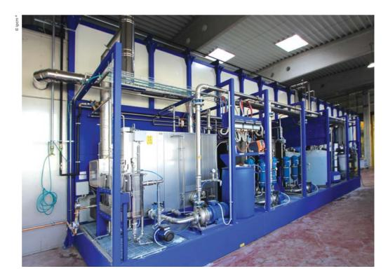
The waste water recovery and filtration skid.
