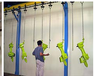
Loading and unloading station
