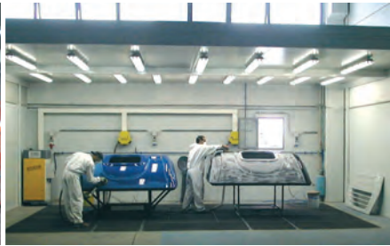
Range for car body with semi-vertical airflow
