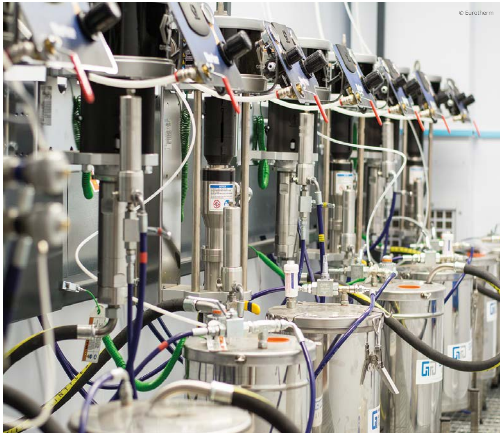
Close up on Graco's Merkur pumps used for the paint supply.
