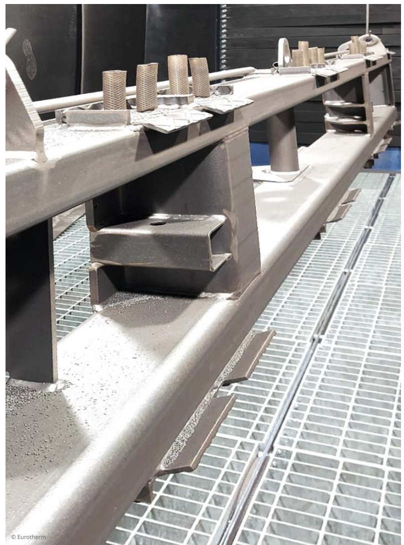
The blowing zone after the shot blasting.
